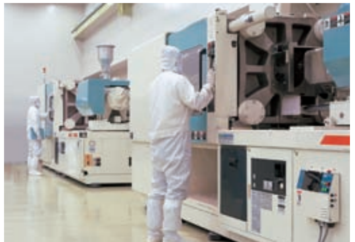
Clean room (injection processing)
